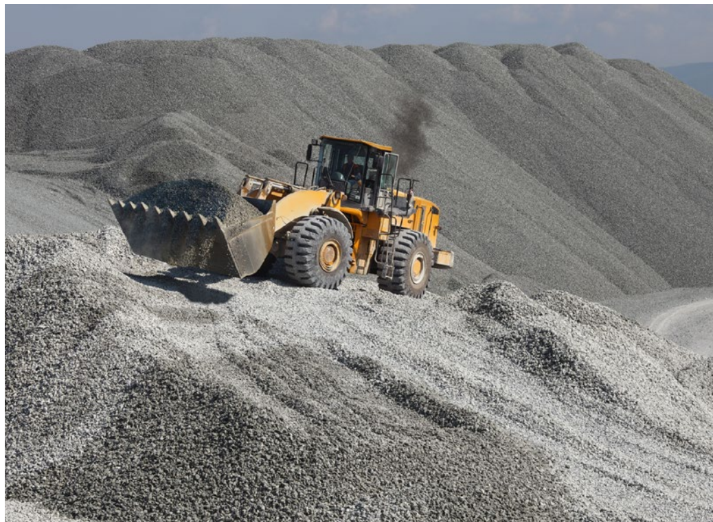
FIGURE 3 The computed surface properties and vehicle speed serve as references to determine when and where to move the bucket (© Salienko Evgenii | shutterstock.com)
