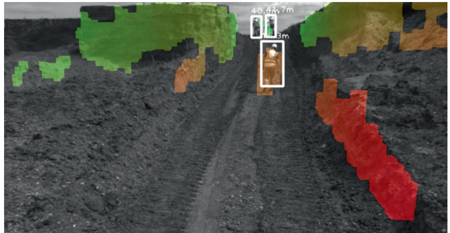
FIGURE 4 Detection of people (obstacles detected are color-coded based on their distance from the camera (green: far away; red: close by); in addition, any pedestrians are marked with a frame) (© ITK Engineering)
