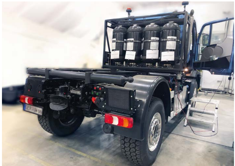
FIGURE 4 The four upright H 2 pressure tanks installed in the body of the Unimog road vehicle (© Daimler Truck AG)
